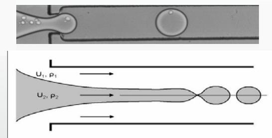
The formation of droplets is due to the interplay between viscous forces and interfacial forces
