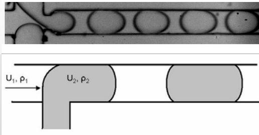
The breakup process is driven by the build-up of pressure upstream of an emerging droplet
